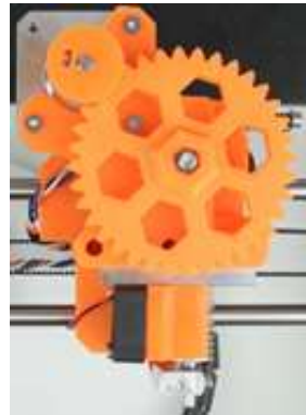
Fig. 12. Example of the geared extruder [11]
