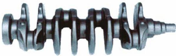
Whether connecting rods, journals, transmission shafts or other closed-die forgings: SMS group's die-former unites traditional forging handicraft with automated industrial manufacture – precisely, productively and cost-effectively. Here are just a few examples from the die-former's extensive spectrum of forging capabilities.
