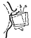
FIG. 42. Influence of tool vibrations on the turned surface (from Kronenberg): — a) normal position of turning tool; - - - b) highest position of turning tool during vibration; - - - c) lowest position of turning tool during vibration; — turned surface.
