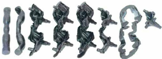
Whether connecting rods, journals, transmission shafts or other closed-die forgings: SMS group's die-former unites traditional forging handicraft with automated industrial manufacture – precisely, productively and cost-effectively. Here are just a few examples from the die-former's extensive spectrum of forging capabilities.
