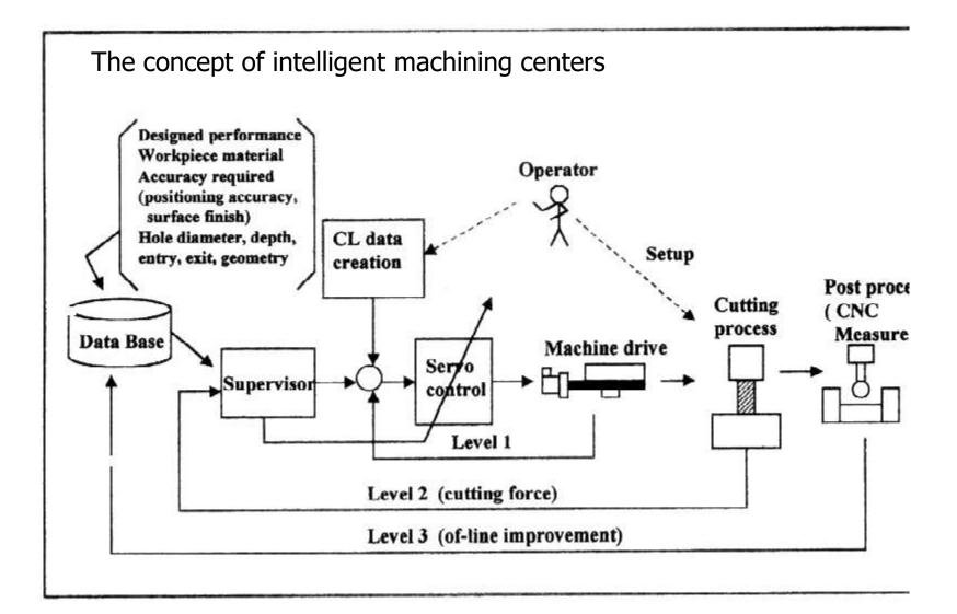
Principle - adaptive control system based on information on the machining process changing cutting conditions.
